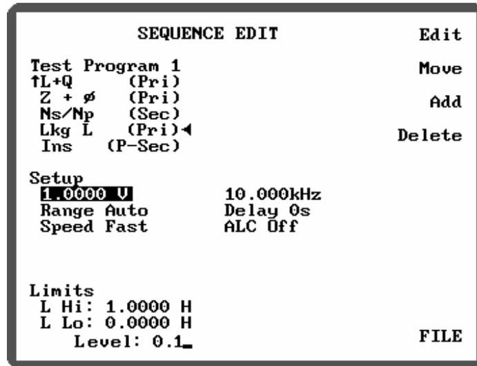
Figure 5-32 SEQUENCE EDIT MODE:Change Test Parameter
