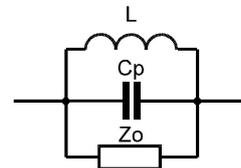
Figure 5-48 Parallel Equivalent Circuit
