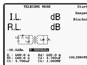
Figure 5-38 TELECOMS MODE: Damped Termination with DC Blocking Capacitor
