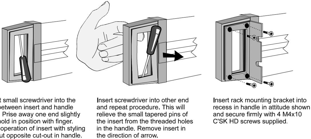
Figure 3-1 Procedure for Attachment of Rack Mounting Brackets
