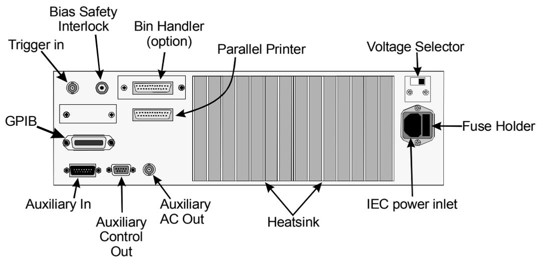
Figure 4-1 The 3260B Rear Panel
